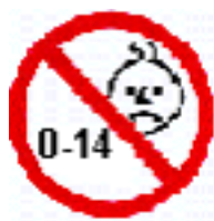
Figure 5.1: Warning symbol : luminaire not adapted to children under 14
